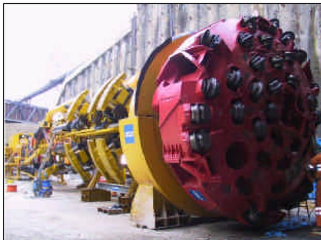
Cutting head of Pilot TBM (5m diameter)
